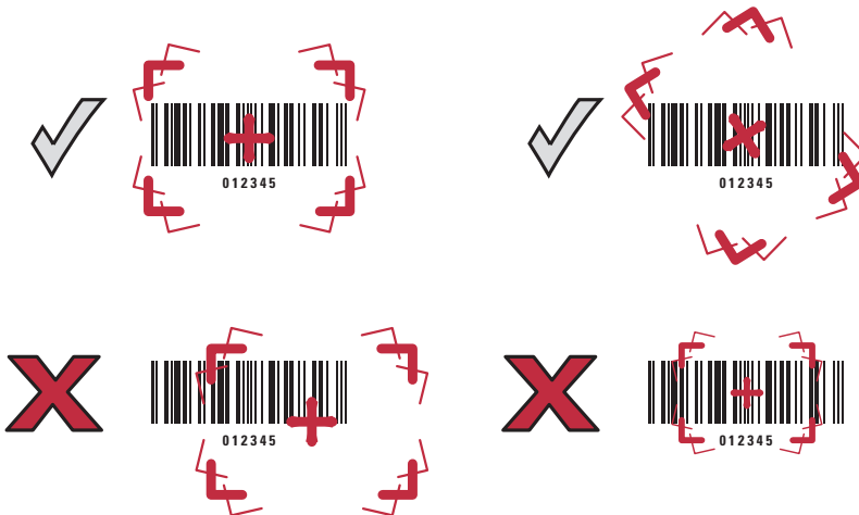
Figure 2-4 Acceptable and Incorrect Aiming - Standard Pattern
